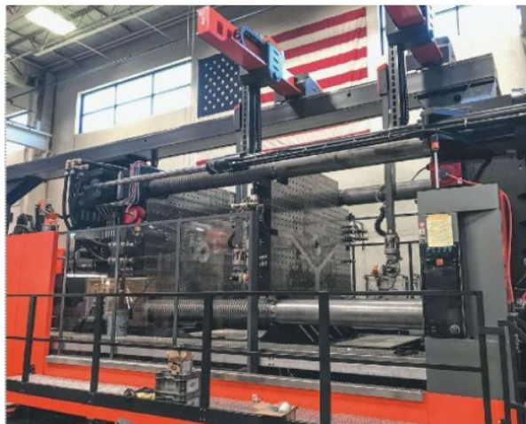
Shape’s newest machine is a 2500 ton Engel combiM press. First shots were expected in early October, with full production in Q1 2020.
